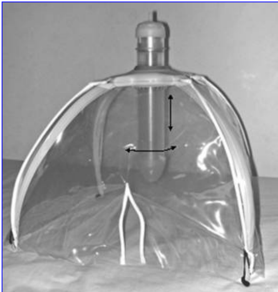
FIG. 1. The nebulizer hood inhaler. The arrows show possible modifications of the funnel.
